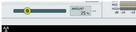
A De-Esser is a compressor type used to reduce only specific sibilant frequencies. Typically the “ss” sounds can be far too dominant on a vocal track and the track would therefore often benefit from being processed by a De-Esser.
