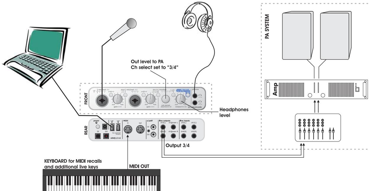
This example illustrates how Konnekt integrates perfectly in a live setup. The objects in a live setup could be:
