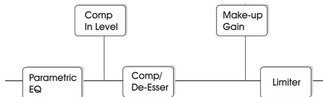
The signal flow in Full-band mode is similar to 3-band mode. The difference lies solely in the Full-band compression as opposed to the split-filter and 3 compression bands found in 3-band mode.
