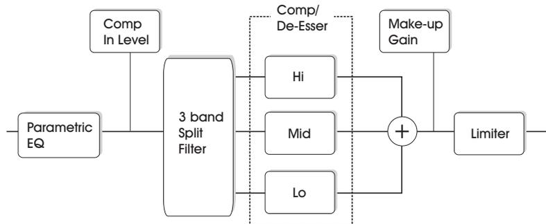
This is a schematic overview of the signals flow through the algorithm in 3-band mode. As illustrated - the signal first passes the 4 band parametric EQ. Then the signal is split into lo-, mid- and hi-bands for individual compression. Cross-over frequencies between the bands are set by the selected Source type. After the Make-up Gain section, the signal passes the Limiter.
