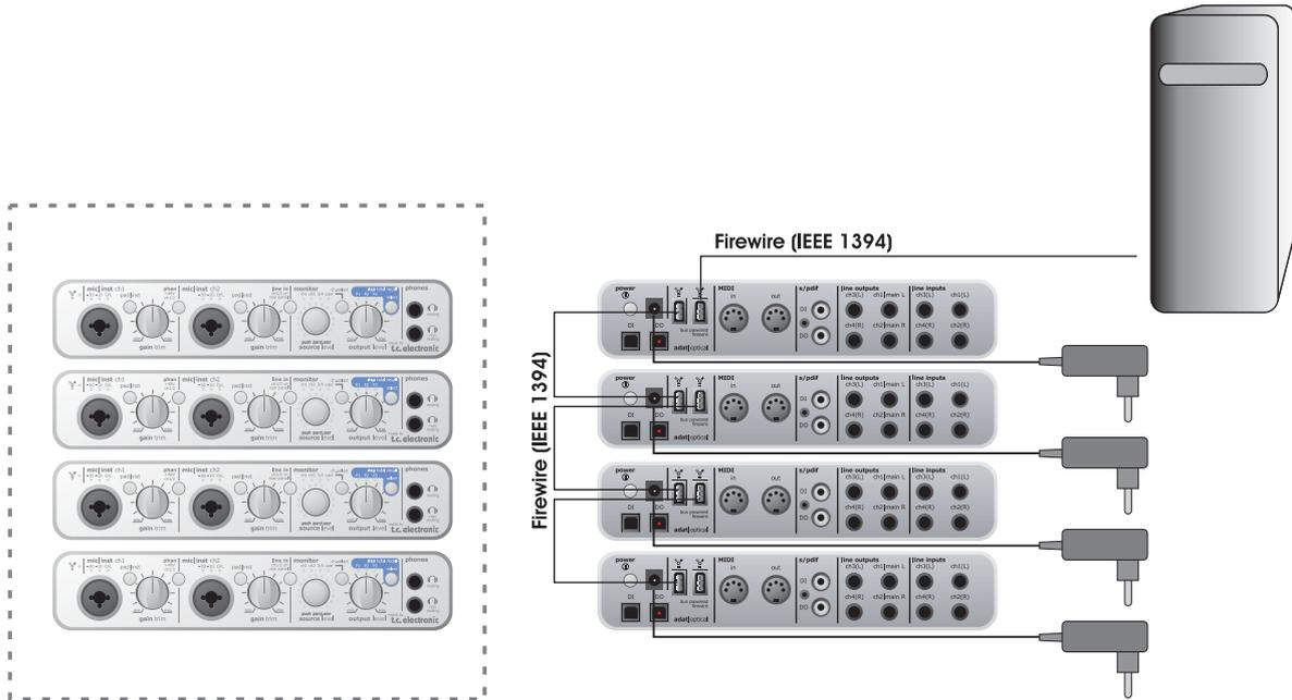
This setup shows how 4 Konnekt 24D units are hooked up via FireWire. With this setup you have up to 4 times as many inputs/outputs as with a single unit.
