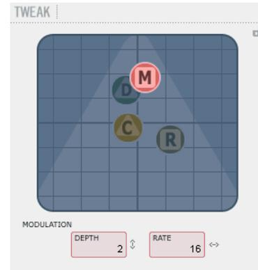
The algorithm designers have adjusted the diffuse field part of the reverb to be as smooth and natural sounding as possible. However, by modulating the diffuse field, the reverb will, in certain cases, integrate better with the entire signal. You may also find the modulation parameters useful simply to create new flavors of reverb.
