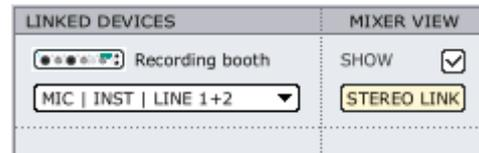
We have labeled the two Konnekts “Control Room” and “Recording booth”. The “Control Room” unit is the unit we have connected to our active speakers, but we would like to listen to the Mic/Inst front panel inputs on the “Recording booth” unit. This is what we have selected via the drop-down menu.
