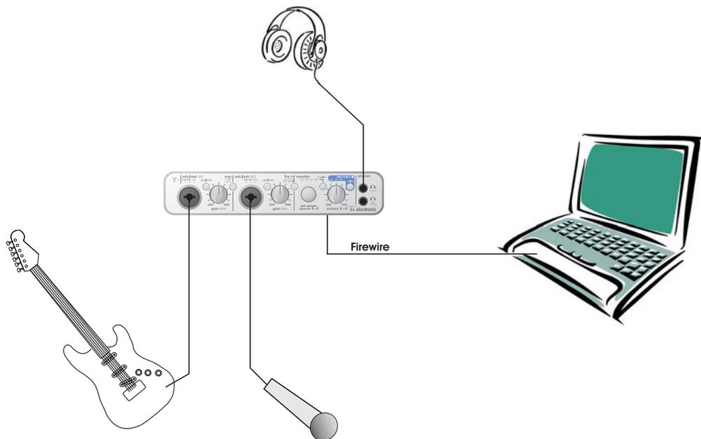
**This is a typical small mobile setup with just a guitar, a microphone and a laptop computer.**
