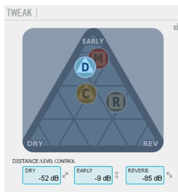
The relation between Dry, Early and Reverb levels defines the perceived distance of a source. The less dry the signal compared to Early and Reverb levels, the greater the perceived distance. Early and Reverb levels set the relation between the amount of room definition compared to the reverb diffuse field.
